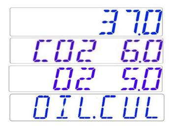
Force scroll between parameters with  $(\Rightarrow)$  key.
