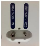
**Figure 11.1** Gas inlets on the back of MIRI® Humidity multiroom IVF incubators
